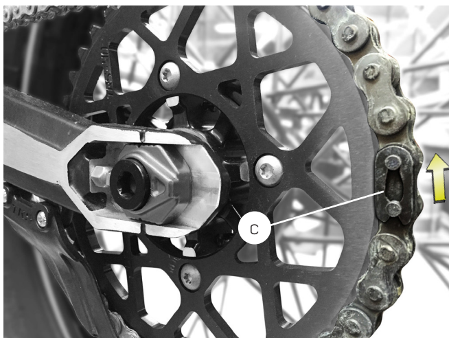
c) Chain Connecting link.
