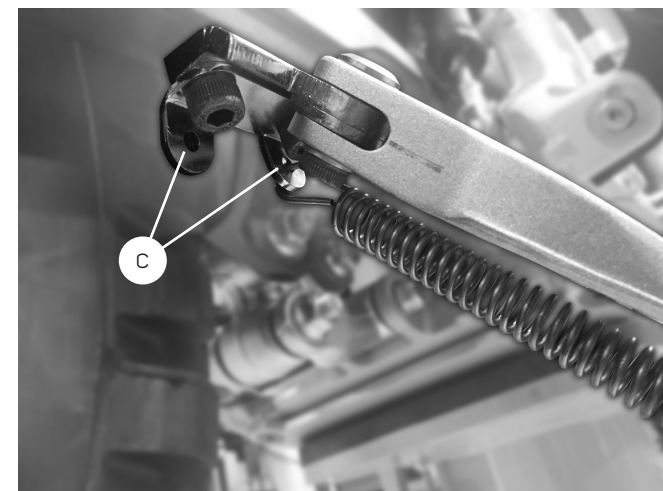
c) Adjustment holes in the side stand
