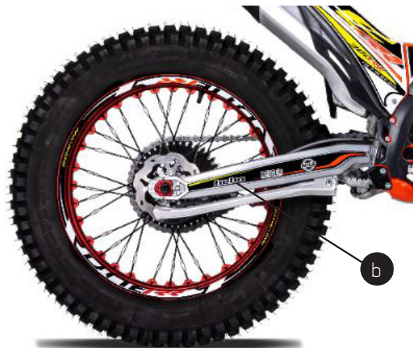
b) Important! The swing arm and the rear suspension need to be regularly maintained.
