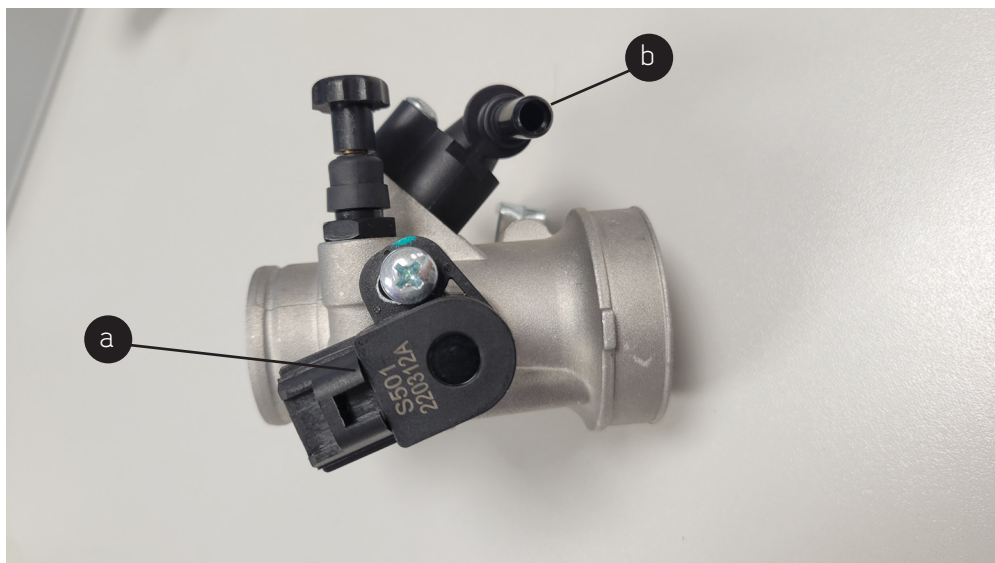
a) Throttle position sensor (TPS)
