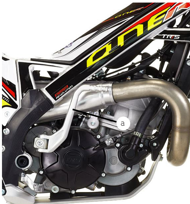
a) Start lever, on the right side of the TRS One
