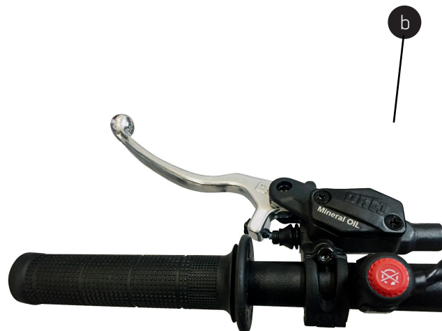
b) Stop button, to the left of the handlebar
