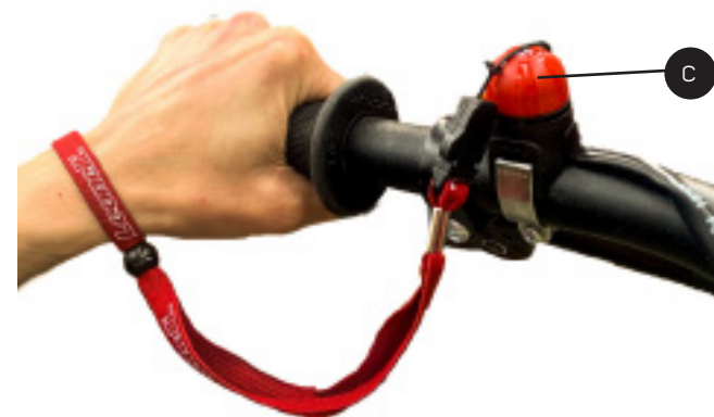
c) Kill switch, to the right of the handlebar
