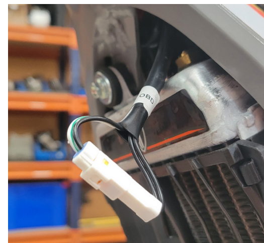
b) Calibration bridge connected.
