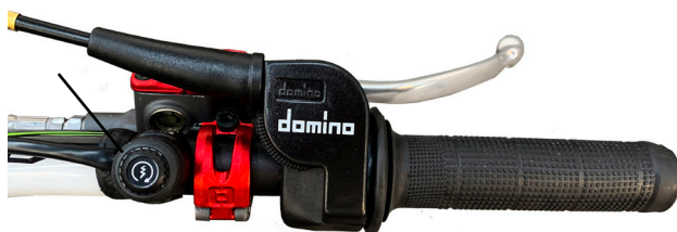
a) Electric start switch button, on the right side handlebar
