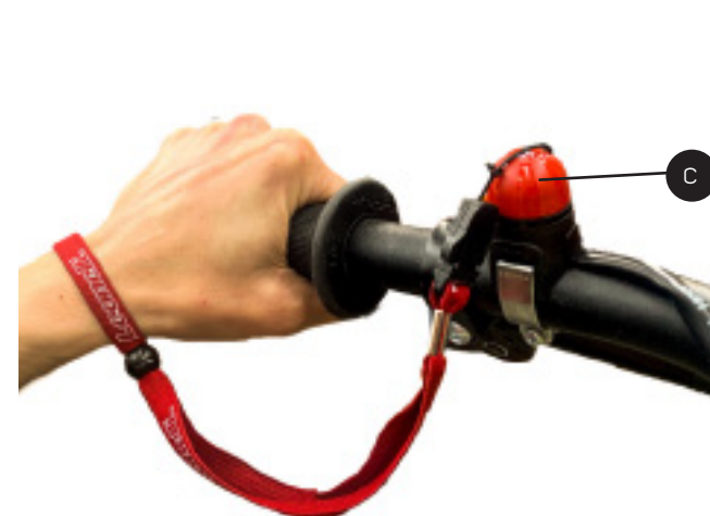
c) Kill switch, to the right of the handlebar
