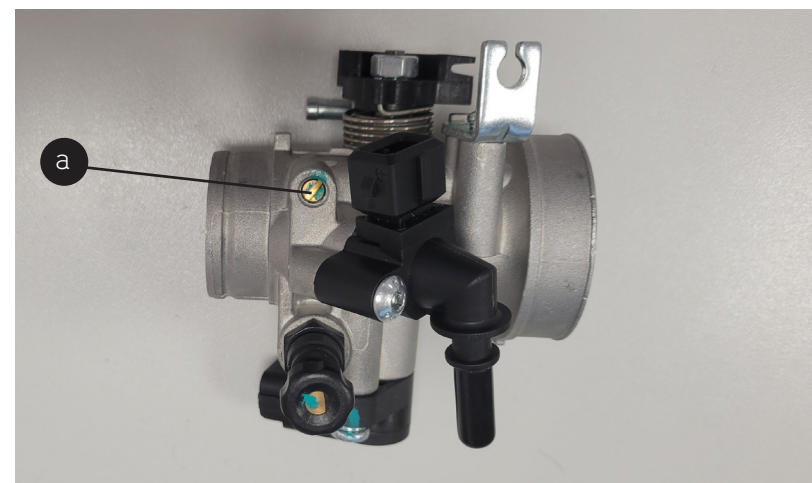
a) Idle speed screw adjuster
