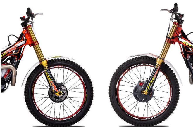
a) Spring preload; b) Compression adjustment
