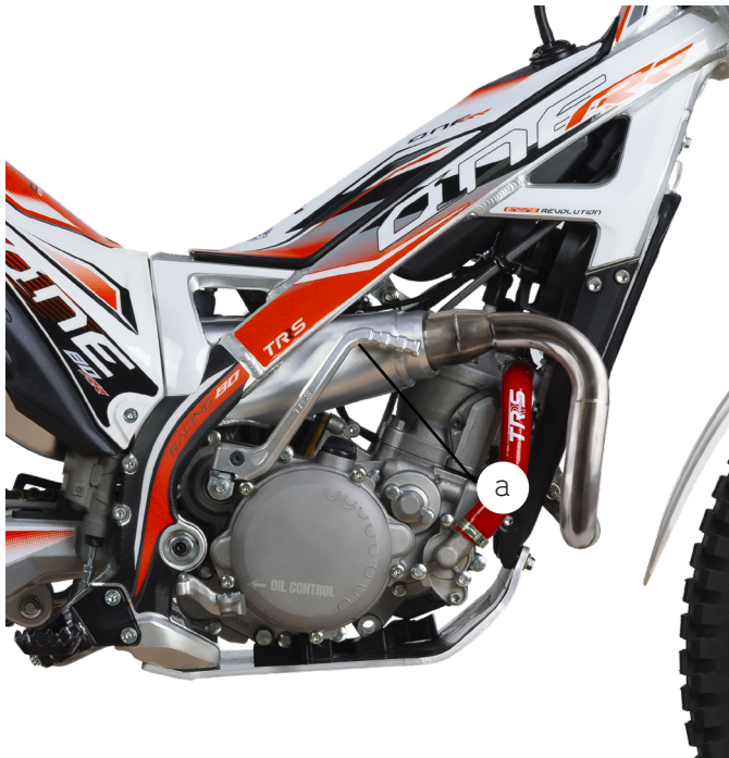
a) Start lever, on the right side of the TRRS RR 80cc
