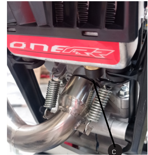
c) Temperature sensor, screwed on the bottom of the radiator.
