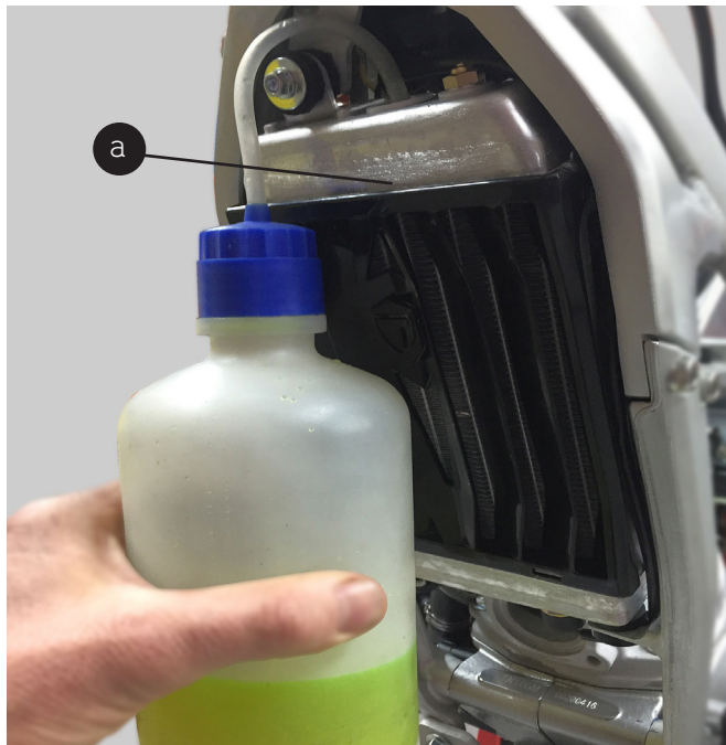
a) Filler cap located on the top of the radiator.
