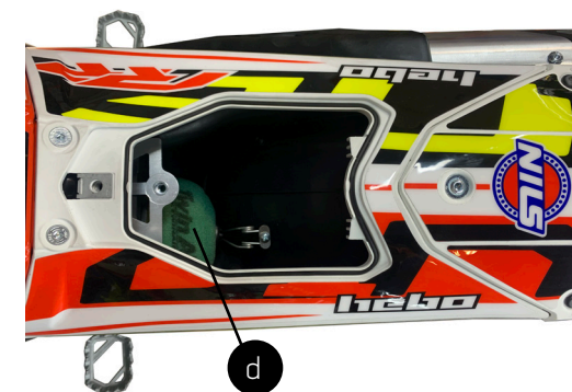
b) Removing the cover, you can access the air box baffle; c) Air box baffle.
