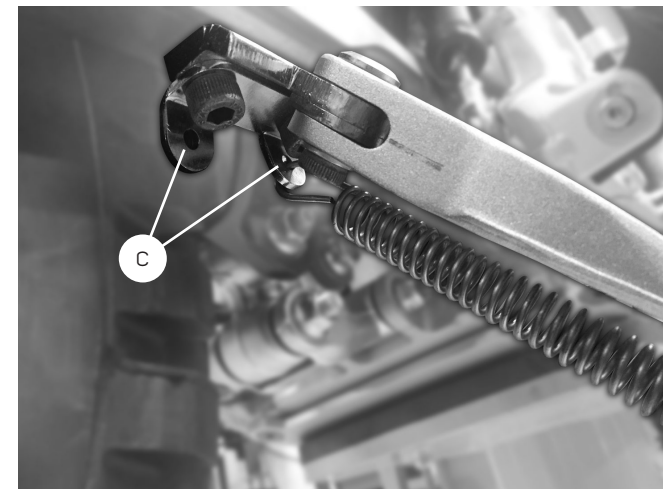
c) Adjustment holes in the side stand
