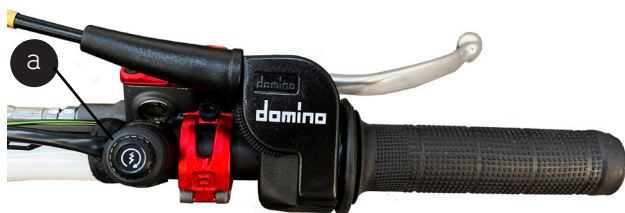
a) Electric start switch button, on the right side handlebar
