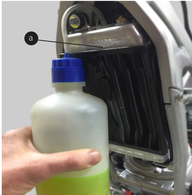
a) Filler cap located on the top of the radiator.
