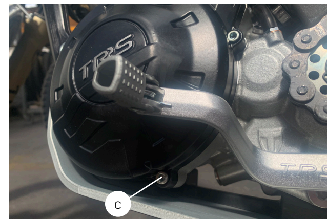
Fig (c): Oil drain plug, remaining oil placed on the electric start cover.
