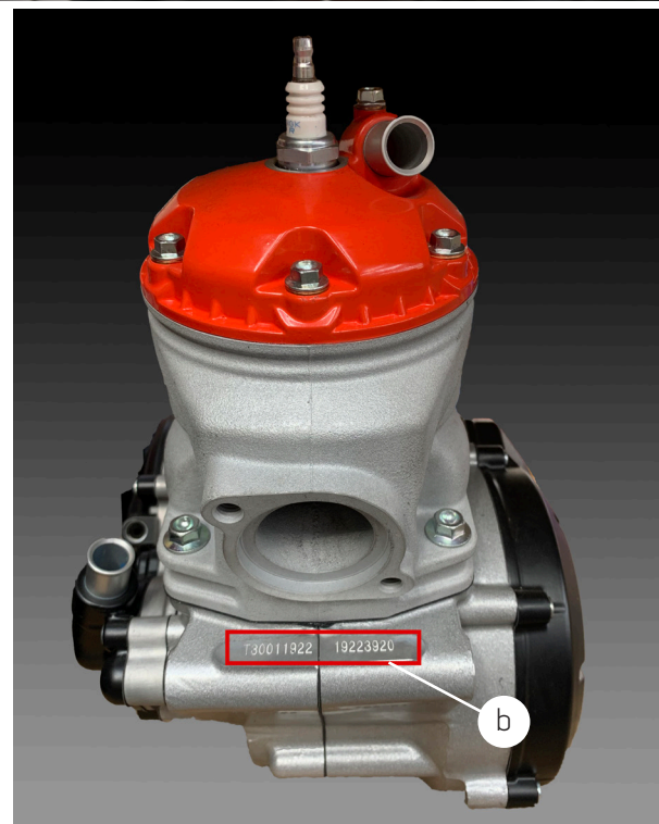
b) The identification number engine, is located under of the exhaust pipe
