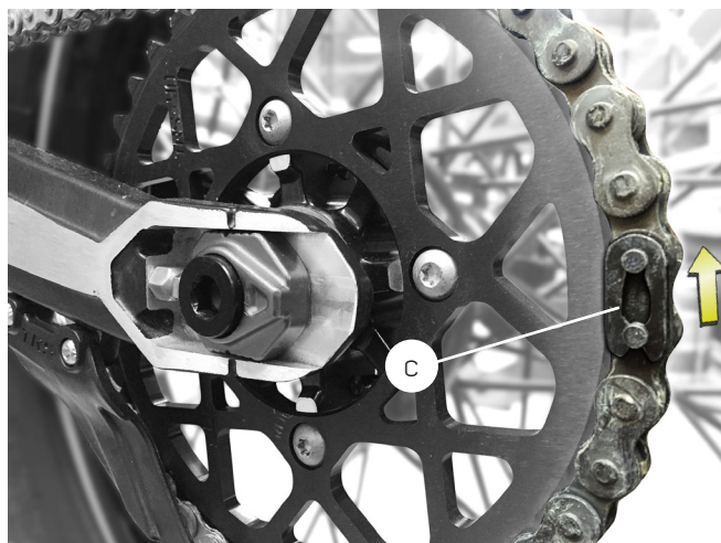
b) Once you have adjusted the chain to the right tension, tighten up the axle.
