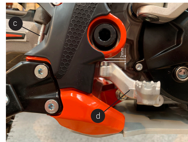
c) Tensioner rod rear brake pedal; (d) Screw for height adjustment of the brake pedal. For correct performance, you need to leave a small clearance gap.
