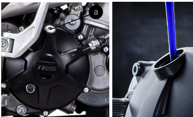
a): Oil filler cap, in the upper part of the crankcase.
