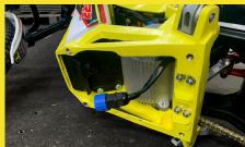
Put your ON-E on the ground and with a 5 mm Allen wrench, remove the 4 screws from skid plate of the chassis and unplug the connector from the battery twisting the lock ring counterclockwise.
