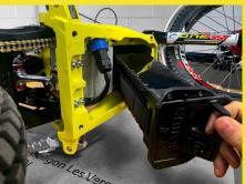
Then remove the screws from the plastic cover battery with a 4mm allen wrench and take off the battery.
