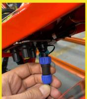
Put in the correct position the two-pin plug (fig F) aligning the white dot with the protrude from the charging connector (fig E). Screwed in the nut that brings the two-pin plug (fig D). Replace the blue cap when the battery is fully charged.
