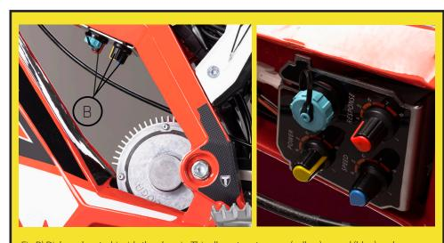
Fig B) Dials are located inside the chassis. This allows to set: power (yellow), speed (blue) and response (red). Turning the adjusters clockwise, the performance of the motorcycle increases. On the contrary direction, turning counterclockwise, the performance is reduced to a minimum.
