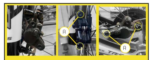
Using the 5mm Allen wrench, loosen the two screws on the front and / or rear brake caliper.
