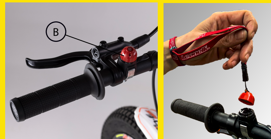
Figure B) Kill switch, put the elastic band on the left wrist
