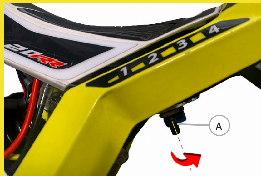
A) Dial adjuster, as we turn clockwise, the motorcycle response will increase, the same happen with speed and the power will be higher.
