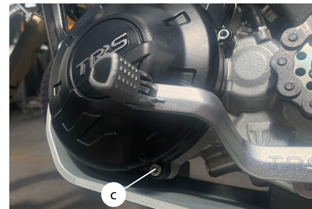
Fig (c): Oil drain plug, remaining oil placed on the electric strat cover.
