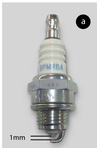
a) The plug that is factory-installed is defined in the technical specifications. Tighten to 11Nm.
