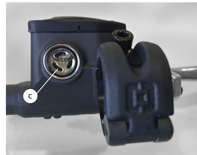
c) Level of fluid in the front brake pump.
