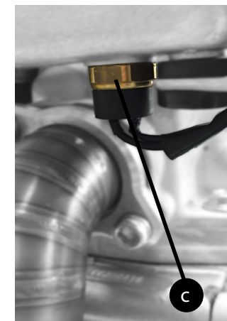
c) Temperature switch located at the bottom of the radiator.
