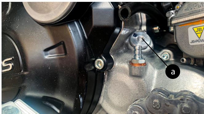
a): Oil filler cap, in the upper part of the crankcase.
