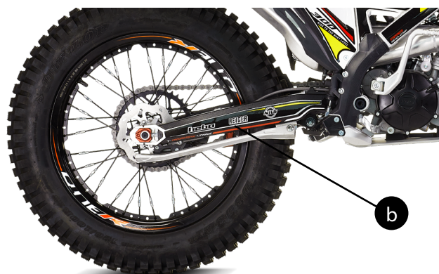
b) Important! The swing arm and the rear suspension need to be regularly maintained.
