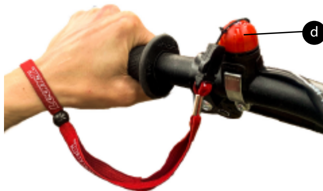
c) Kill switch, to the right of the handlebar
