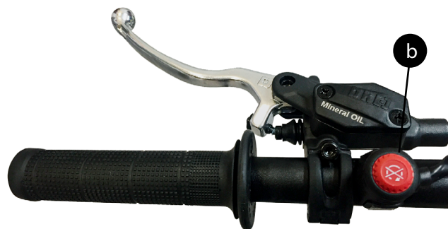
b) Stop button, to the left of the handlebar
