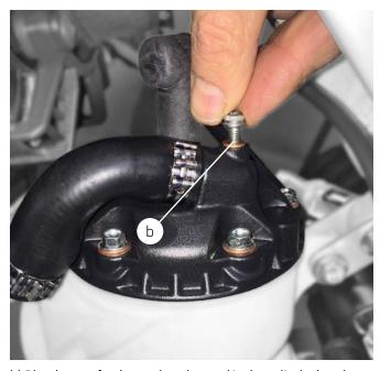
b) Bleed screw for the coolant, located in the cylinder head.
