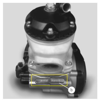
b)) The engine identification number, located under the reed valve of the carburettor.
