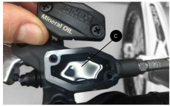
c) Clutch pump tank. Only mineral oil may be used, in order not to damage the o-rings
