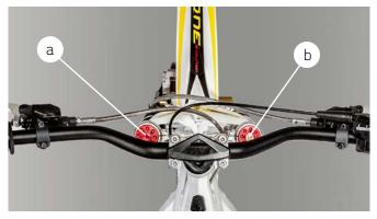
a) Spring preload; b) Adjusting the length
