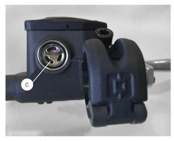
c) Level of fluid in the front brake pump.
