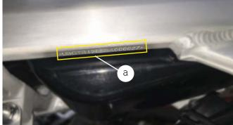
a) The position of the identification number, located on the tube on the right hand side of the frame.
