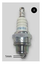
a) The plug that is factory-installed is defined in the technical specifications. Tighten to 11Nm.
