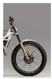
a) On the right-hand side of the suspension you can set the preload.
