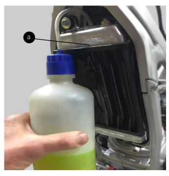
The factory-supplied coolant is a permanent-type antifreeze of ethylene glycol, diluted in 50% distilled water and containing anticorrosive additives.
